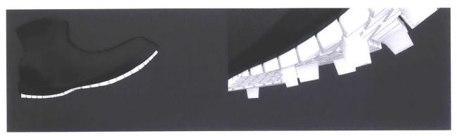
Figure 68. Illustration showing the application of Exoskin as the sole of an active shoe. Left: default state, Right: actuated state.
