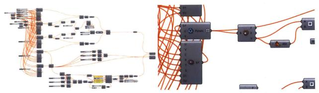
Figure 47. Screenshots showing Grasshopper script written to create the triangular panelization architecture on a given surface
