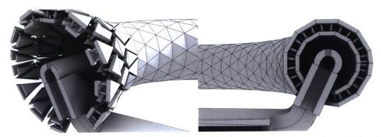
Figure 66. Close-up illustrated views of the molding architecture, panelization, and spoke structure of the prototype design.
