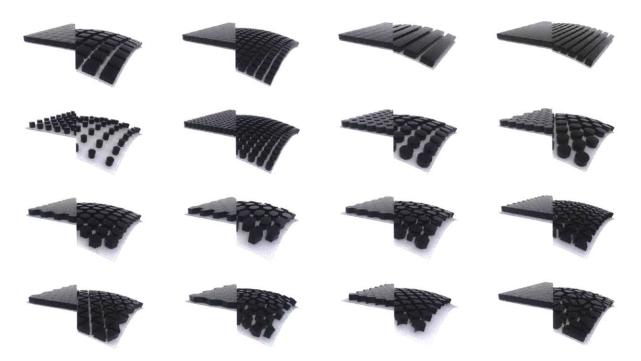
Figure 31. 3D visualization of the panelization methods from Figure 30 including quad meshing, triangular, hexagonal, voronoi, and more. Shown here are the default and actuated states of each.
