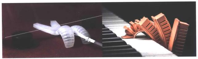
Figure 13. Left: The soft robot can wiggle its way underneath a pane of glass just three-quarters of an inch above the surface. Right: Four soft robotic fingers progressively curl to play notes on a keyboard.
