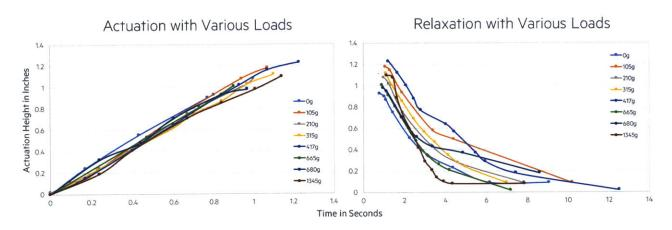
Figure 54. Exoskin composite actuation and relaxation tests under various loads up to about a kilogram.
