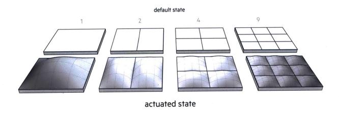
Figure 35. Illustrated diagram showing the tradeoffs between discretization of the bladders and overall actuation amount
