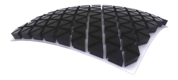
Figure 46. Rendering of the matched triangular panelization pattern on a stretched elastic layer
