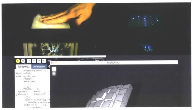
Figure 6. Pneuxel is made of five by five individually controllable cells that can light up through an optical waveguide composite. It can simulate variable degrees of expansion and contraction through pneumatic actuation. Shown here is the device and software implementation.
