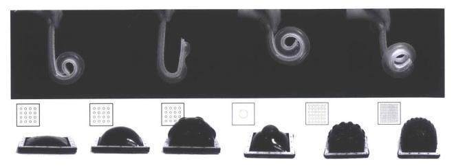
Figure 5. Top: Pneui bending shape primitive. Bottom: shape primitive of multi-stage texture change
