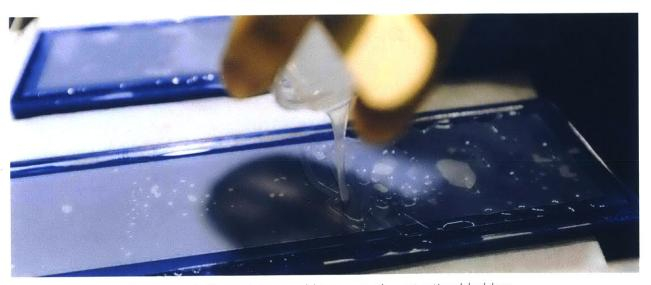
Figure 19. Pouring the uncured silicone into a mold to create the actuating bladders
