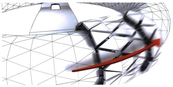
Figure 62. Illustration showing more fine-grain finger-by-finger actuation of Exowheel when communicating the next turn during navigation mode.
