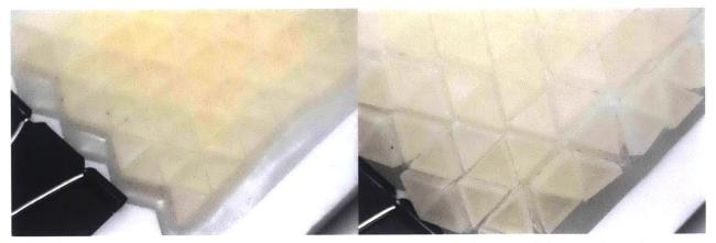
Figure 49. Close up photograph showing the default un-actuated (Left) state of the initial Exoskin prototype and (Right) the actuated state
