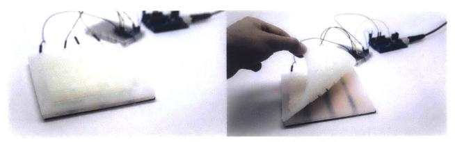
Figure 41. Copper-based capacitive sensing layer prototype with Arduino platform
