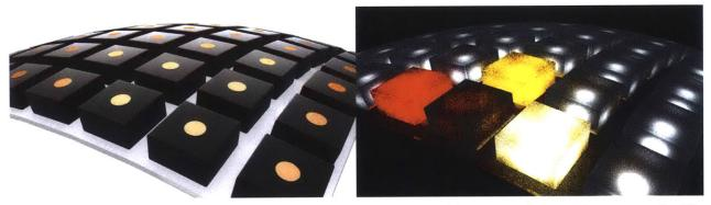
Figure 39. Rendered illustration depicting integrating into the rigid layer, metal capacitive sensors (Left) and integrating LED's for input & output.
