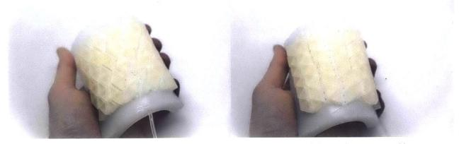
Figure 50. Anisotropy seen in deformation. Flexure in the Y axis caused the scales to group like diamonds (Left) while flexure in the Z axis caused them to group in rows (Right).
