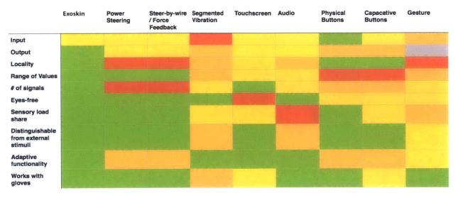
Figure 60. Chart comparing various input and output mechanisms used in automotive steering wheels
