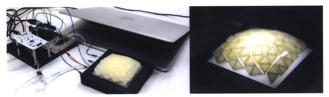
Figure 53. Combined prototype with capacitive sensing, embedded LED, and actuation all on dynamic feedback loop controlled by both an Arduino and Pneuduino.
