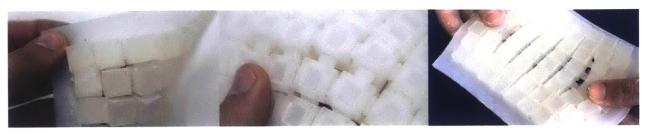
Figure 45. Exoskin composite prototype photographs showing the thin silicone connective tissues inbetween the scales.
