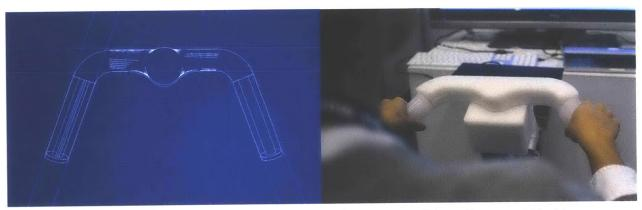
Figure 17. Left: Technical sketch of Focal Wheel design showing overall form factor and bladder placement. Right: Final Focal Wheel prototype during member's event
