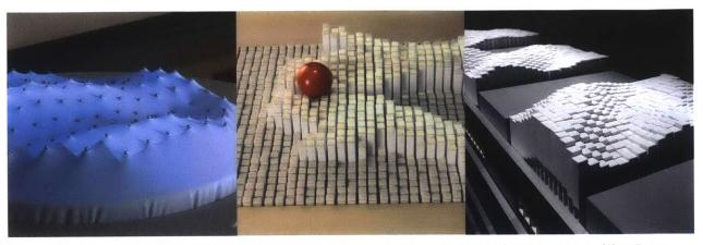
Figure 11. From left to right: (1) Relief: low-density shape display with latex sheet covering, (2) inForm: higher-density display capable of representing human-scale features, and (3) TRANSFORM: design-lead piece able using motion to depict waves & other non-rigid modalities
