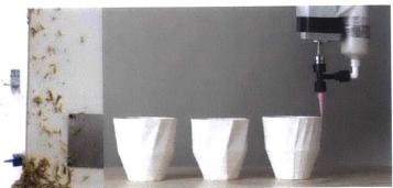
Figure 27. Left: 5-axis CNC milling of a wooden block using a KUKA Robotics arm to create a complex form. Right: Antwerp-based design studio Unfold 3D printing ceramic using their proprietary method.
