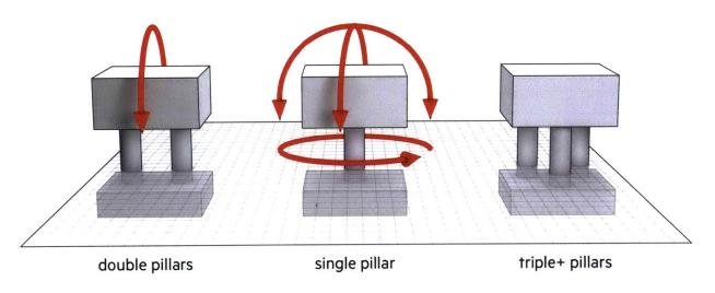
Figure 44. Illustration showing the degrees of freedom of movement for an individual rigid scale depending on the number of pillars.
