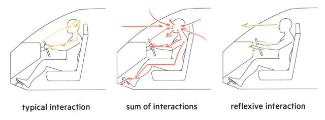
Figure 59. Diagram showing the progression from a typical automotive interaction loop requiring a glance at the dashboard to an evolved reflexive interaction loop allowing the hands to bypass the eyes.
