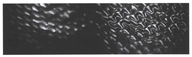
Figure 22. Macro photographs showing the texture change using the Biologic natto cells on latex. The left photograph shows their humid state, while the right photograph shows the arid state.
