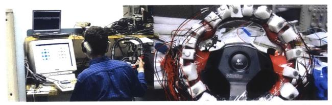
Figure 57. Left: Enriquez's tactile wheel that provides haptic feedback to alert the driver of a possible problem. Right: Haptic steering wheel developed by AT&T using 20 vibration motors.
