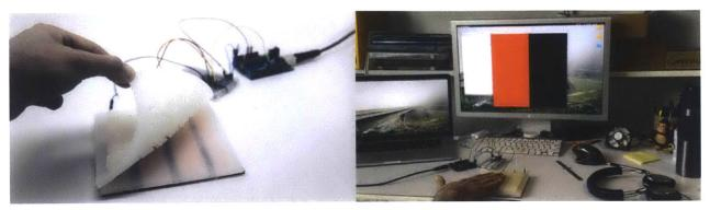
Figure 52. Copper-based capacitive sensing layer prototype with Arduino platform
