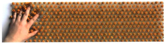
Figure 10. Super cilia skin is a tangible interface which responds to touch. Like our skin, it is a haptic I/O membrane that can sense and simulate movement and wind flow.
