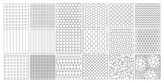
Figure 30. Variety of 2D panelization methods explored in early Exoskin samples including quad meshing, triangular, hexagonal, voronoi, and more.
