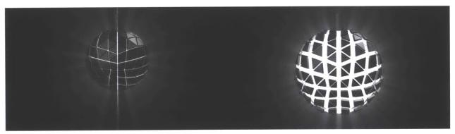
Figure 71. Illustration of opaque Exoskin rigid material with interior light source and dense panelization method in order to create a dimmable lamp. Left shows the default state while Right shows the inflated, actuated state.
