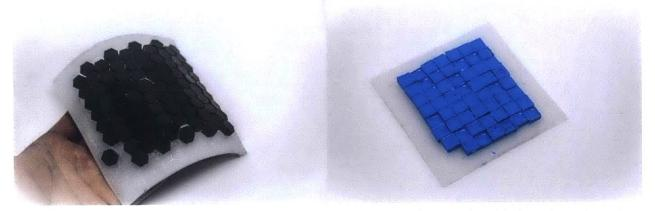
Figure 43. Left: Lasercut acrylic scales epoxied to silicone sheet. Right: Hand-molded urethane-based resin plastic square scales epoxied to silicone sheet.
