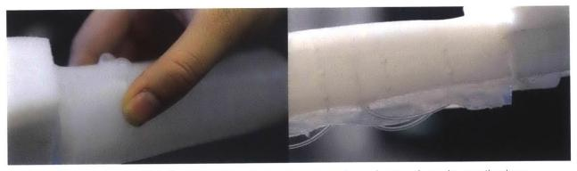
Figure 18. Over-actuated smaller air bladders in top layer in order to better show the tactile shape change happening underneath the palms during GPS turn navigation
