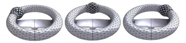
Figure 65. Illustration of final fully-panelized design for Exowheel showing the medium-sized bladders actuating clockwise around the rim.
