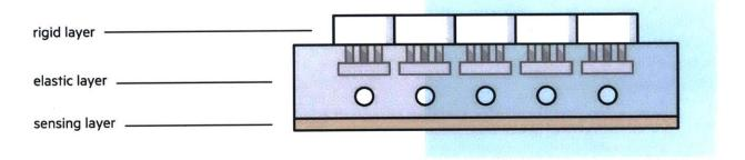
Figure 23. Simplified illustrated diagram showing the three key layers in Exoskin
