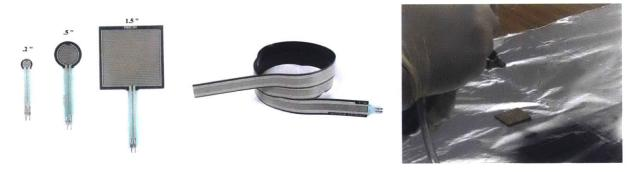
Figure 40. Left: variety of pre-fabricated force resistive sensors available off-the-shelf from sites like Sparkfun and Adafruit. Right: Applying FSR ink to a surface using an airbrushing system.
