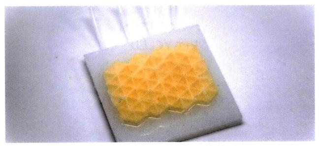
Figure 51. Same triangular panelization method now with 4 discrete bladders in rows
