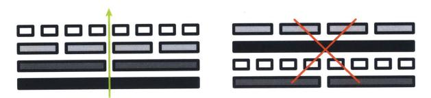
Figure 37. Illustration showing the correct, ascending order for actuated bladders in the elastic layer
