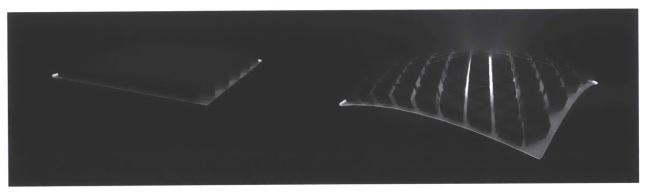
Figure 32. Visualization of triangular panelization scheme applied to an opaque rigid layer embedded in Exoskin. Placing a light source below reveals the high control of permeability this scheme enables.
