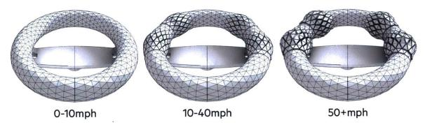
Figure 61. Illustration showing dynamic reaction to changes in speed and hand placement. As speed increases, the grip more tightly cups the drivers hands for safety and comfort.
