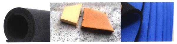
Figure 28. Left: Wool felt. Center: Two pieces of raw leather hide Right: Blue neoprene rubber fabric.
